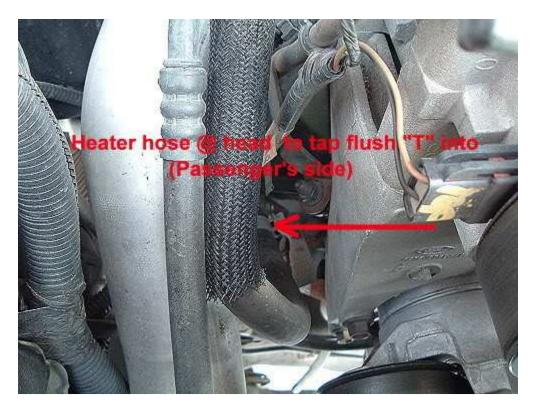
Install that heater hose to one end of the 5/8" flush "T".
