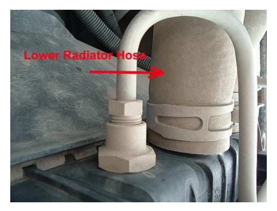
Remove driver's side block plug with 1/4" socket wrench driver, and drain coolant into suitable container.
