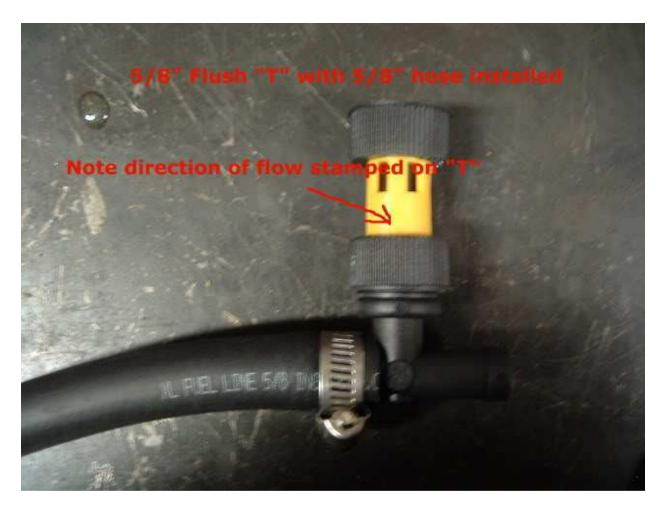
Install the remaining end of the 5/8" hose to fitting where the original hose was removed from the engine.
