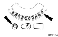
3. Inspect the bearing for brinelling (surface indentations in the raceway).
