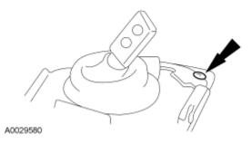
4. Remove the lower gearshift and shift housing.
